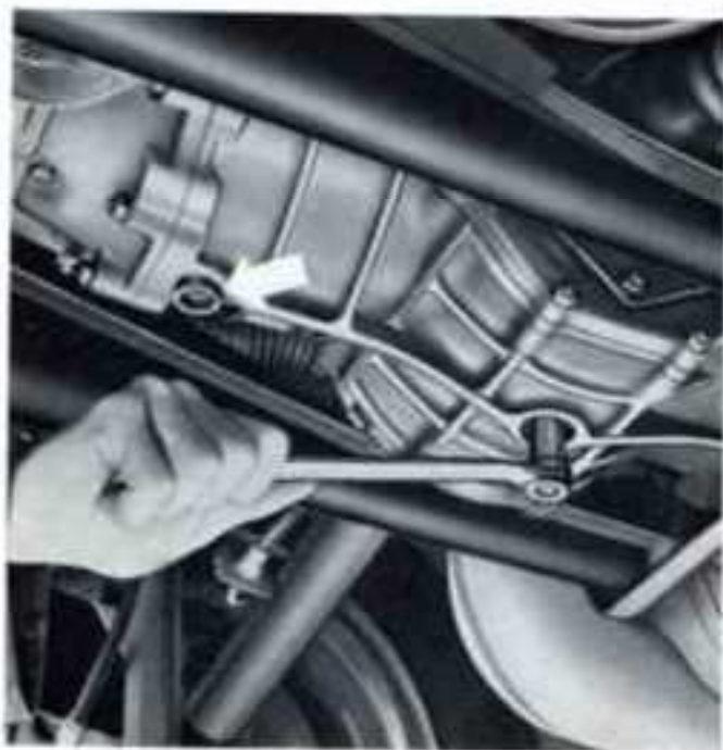
Draining the transmission oil
