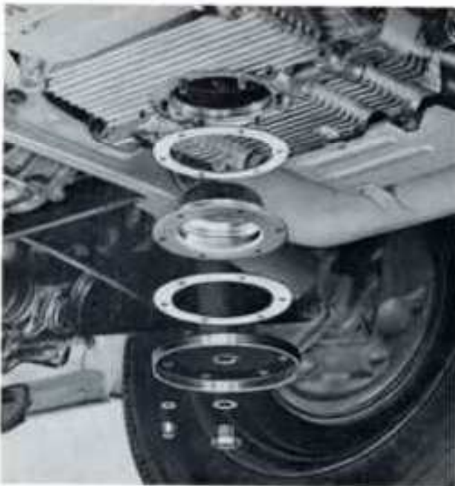
Cleaning oil strainer
