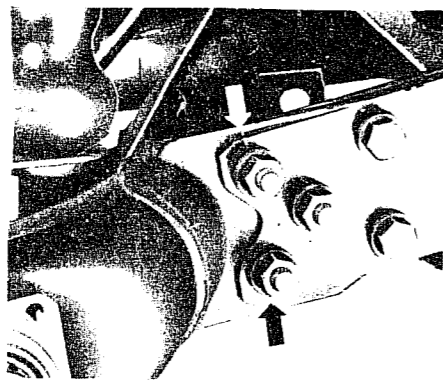
Fig. F.21. Mark the relative positions of the spring plate and the trailing arm before disassembly - D/J axle.
